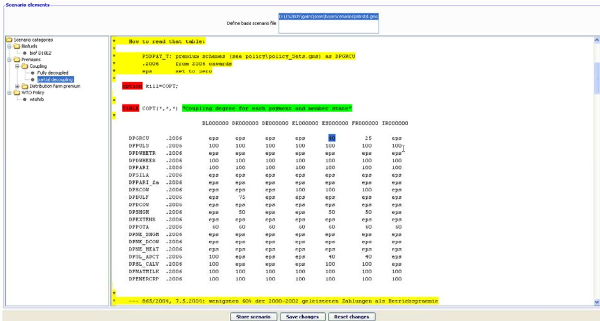
Storing the scenario then generates a file as shown below, user name, the reference to CAPMOD.GMS and the date and time are automatically added by the GUI. The files will be added to the files stored in “gams\pol\_input”.
